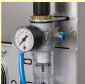
Forced cooling system with compressed air
