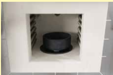
Loading in the sintering furnace LT 02/13 CR
